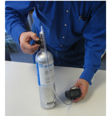
Figure 1: Performing a functional “bump test” by exposing the instrument to test gas takes only a few moments perform.
