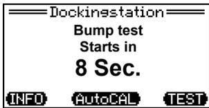
Bump test starts after 10 seconds automatically
