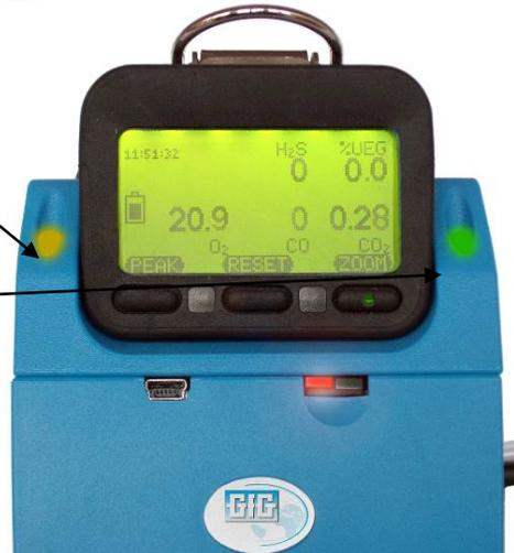
The normal charging process of an empty battery takes approximately 7 hours. After the normal charging process, the detector automatically changes to a trickle charge.
