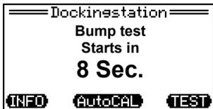
Bump test starts after 10 seconds automatically
