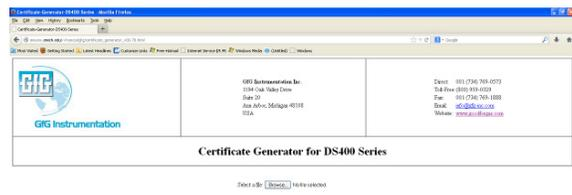
To generate a certificate, a TS400 file must first be opened. A TS400 file is a data file from the TS400 SD memory card. Click the **Browse** button and select the TS400 file from the location where it was stored on the computer. Once the file is opened the fields on the Certificate Form will be populated with the data from the first record in the data file.
