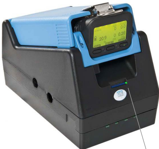
Bump test successful: Display is green + green LED lit in slot
