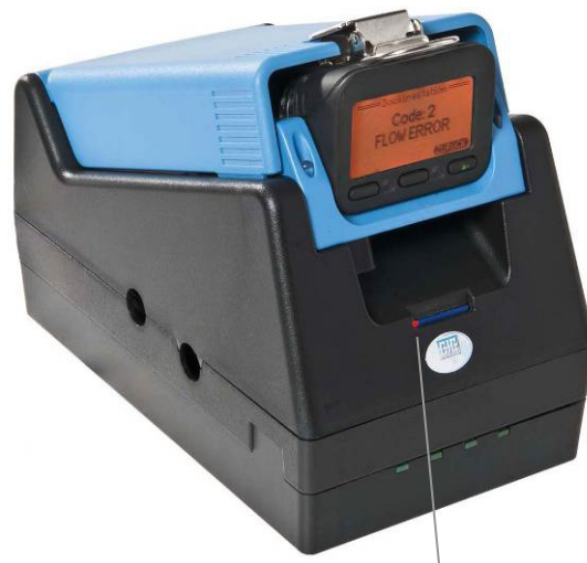
Calibration failed: Display is red + red LED lit in slot Display of the error which has occurred (shown here Code 2: Flow error)
