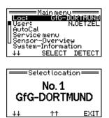
From a table stored in the device, it is possible to select one of 100 possible places. All table entries can only be edited with a PC. In a table entry it is possible to save up to 15 letters / figures, which are saved as "**Job site**" in the G888.
