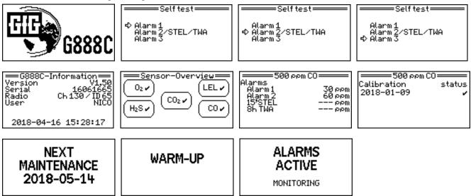
Alarm thresholds and calibration data will be displayed for all available sensors. Please find an example of CO below. Depending on the condition of the sensors, other messages will be output, which possibly need to be acknowledged. Please find more detailed information in the section "Other messages when starting the device".
