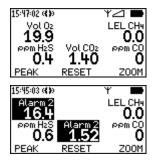
On the left in the picture, the alarm is triggered by a high CO2 reading. In addition to the inverted display alternates "Vol CO2" / "Alarm 2".
