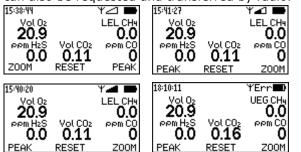
If the radio module is activated, the icons T = 1 for radio and field strength are displayed in the upper display row. The stronger the field strength icon = 1 = 1 and is filled in, the better is the radio connection. A flashing field strength icon = 1 signalises that currently no measured values are requested or that the radio connection is interrupted. If the icon TErr is displayed, the radio module is either defective or switched on but not existing at all.
