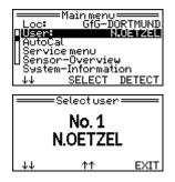
From a table stored in the device, it is possible to select one of 20 possible entries. All table entries can only be edited with a PC. In table entries it is possible to save up to 15 letters / figures, which are saved as "**Identification**" in the G888.
