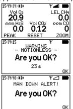
If the device user cannot act for himself any more, he can rapidly call for help by the acoustical alarm signalling or by radio.
