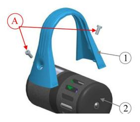
1) Loosen the screws "A" and remove the retaining bracket (1). To do so, slightly pull apart the ends of the bracket until the lugs are free.
