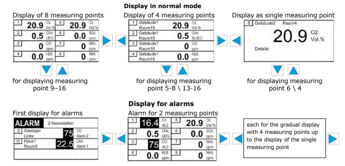
The display is backlit; the light intensity can be increased using any control button. In the event of a gas alarm or faults, the display lighting is automatically activated with a red background.
