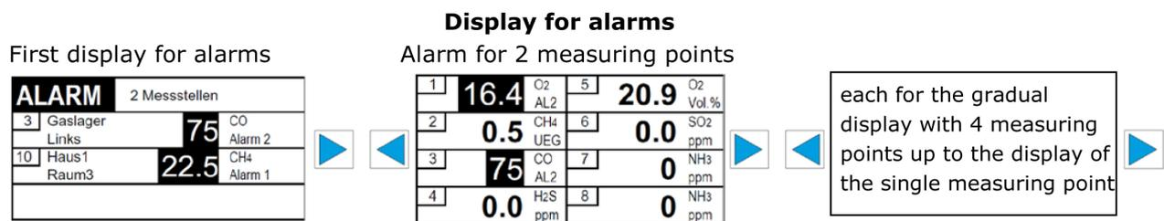
The display is backlit; the light intensity can be increased using any control button. In the event of a gas alarm or faults, the display lighting is automatically activated with a red background.
