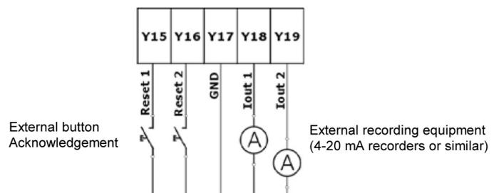
This type of input must be connected to GND to acknowledge alarms.
