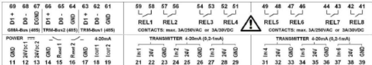
The top terminal assignment applies to the GMA 200-MT6 and the bottom terminal assignment applies to the GMA 200-MT16.
