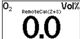
In the third phase, the EC22 has acquired a stable minimum zero gas signal.
