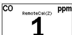
In the second phase, the EC22 has acquired a stable minimum zero gas signal. It displays the text "RemoteCal (Z)" above the measured value. The yellow LED also pulses twice every 5 seconds, with a slight delay.
