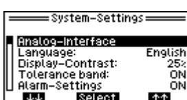
The **Tolerance band** can be "ON" or "OFF". When set to "ON" (default), minor signal deviations from zero gas are displayed as 0 ppm or as 0.0 % LEL. The actual measured value is only displayed when the measured values exceed or fall below the tolerance band. If set to "OFF", the device will always display the actual measured value.
