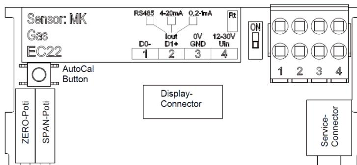
For digital data transmission via RS-485, the bus cabling depends on various factors. This includes the structure of the bus as a string or as a ring, the number of transmitters on the bus, the distance of the individual transmitters from the controller, the transmitter type/model, the sensor type and,
