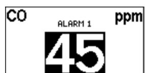
An alarm is triggered as soon as the gas concentration exceeds or falls below the set alarm threshold value. Depending on the function setting, threshold alarms can either be reset automatically or, if the latching function is active, by pressing the button to acknowledge it after the measured value has fallen back below (or has exceeded) the threshold value.
