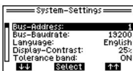
If the transmitter has a RS-485 bus interface, then the **Bus-Address** can be set anywhere between 1 and 247 (0=inactive). A bus address may not be used more than once in the same bus segment.
