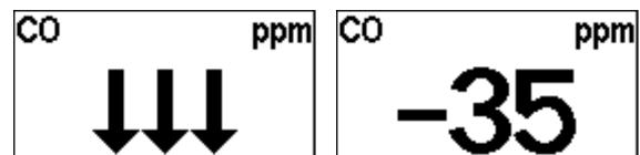
If the measurement signal falls below the value of -7.5 %, the arrows ↓↓ are displayed permanently.
