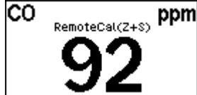
In the third phase, the EC22 has acquired a stable maximum test gas signal.
