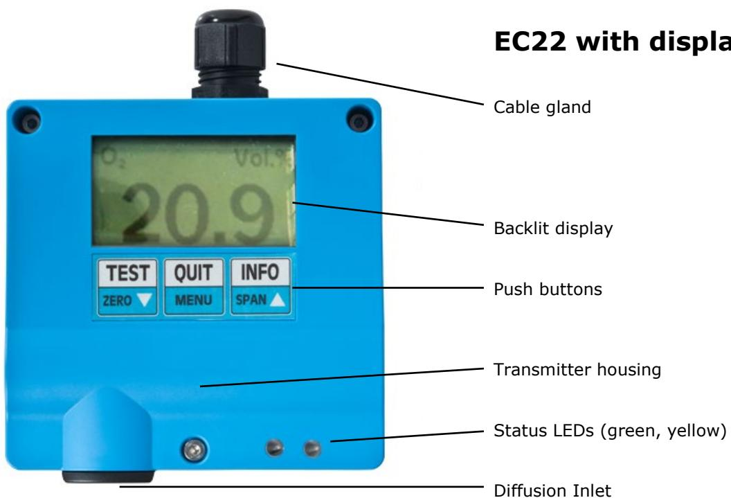
The transmitter housing contains the gas sensor and the transmitter electronics. The electronics converts the measuring signal into a gas concentration which is then signaled via an analog current signal of 4-20 mA or 0.2-1 mA or a digital RS-485 bus signal using the Modbus RTU protocol. In the display variant, gas concentration and status information are displayed.
