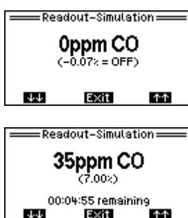
The readout simulation, allows you to test the output signal interface, the measured value transmission and the downstream signal processing. If available, the alarm thresholds can also be checked. The simulation lets you temporarily generate measured values without using a corresponding test gas.
