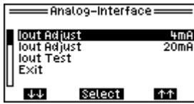
**Iout Adjust:** Caution! The adjustment of the current interface may only be carried out with the aid of a very accurate current measuring device.
