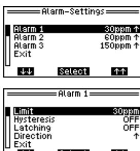
**Alarm1 to Alarm3:** Select the alarm threshold value you need to configure.
