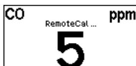
In the first phase, the EC22 displays the text "RemoteCal ..." above the measured value. The yellow LED also pulses once every 5 seconds.
