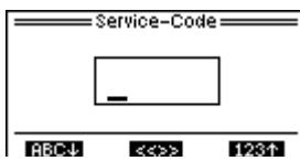
You will have to enter an access code to access the service menu. For the standard service menu this code is "1100". Additional functions are available in an extended service menu. Access to this extended service menu is reserved for GfG service personnel only.
