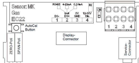
If you release the button during the first phase, which would be too early, no adjustment is made and the transmitter continues measuring as usual.
