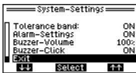
**Alarm-Settings** activates the alarm function and the associated service menu for alarm configuration.
