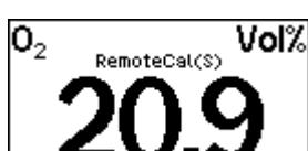
In the second phase, the EC22 has acquired a stable maximum test gas signal. It displays the text "RemoteCal (S)" above the measured value. The yellow LED also pulses three times every 5 seconds, with a slight delay.
