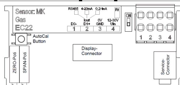
Press the button for at least 10 seconds to prepare the adjustment.
