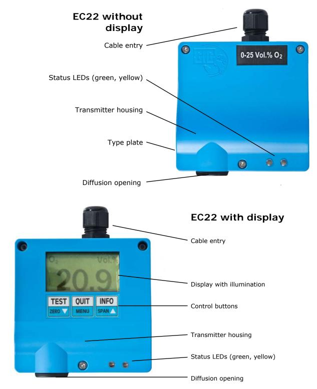
The gas sensor and the transmitter electronics are installed in the transmitter housing. The electronics transforms the measurement signal into a gas concentration and this is signalled with an analogue current signal 4 - 20 mA or 0.2 - 1 mA or digital RS485 bus signal using the MODBUS RTU protocol. Gas concentration and status information are displayed in the display variant.
