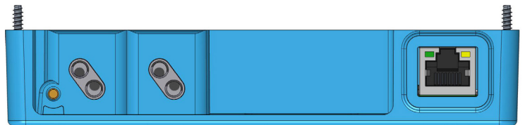
D-ReX housing cover interior view, with LIM
