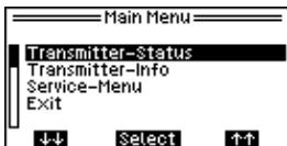
Current system errors, errors in the measurement procedure, service needs and incidents can be retrieved in the transmitter status. Numbers inside parenthesis can be found after these groups. These numbers indicate the number of the existing information.
