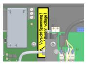
Cables with AC voltages that are dangerous to touch, e.g. 230 V, and cables with non-dangerous DC voltages, e.g. 24 V, must be laid separately from each other. The cables used must be suitable for the intended purpose.
