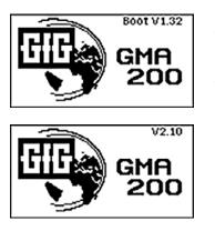
At system start the GfG logo, the device name and first the version number of the bootloader and then the version number of the mainboard firmware is displayed. During this time, various internal self-tests are performed. After completion of the internal tests, a short test of the display, all LEDs and the horn is performed. During the entire time, the yellow "FLT/GMA" fault LED is lit and the relays are de-energized.
