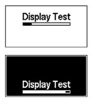
After switching on the device, a test of the display starts automatically. This test can be triggered manually here. If any defects are detected, replace the unit.
