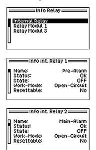
At Info Relays information about the 8 internal relays and eventually connected relay modules can be retrieved.
