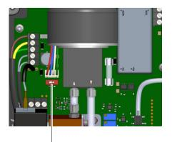
*Switch S5 on the circuit board for switching the pump off and on*
