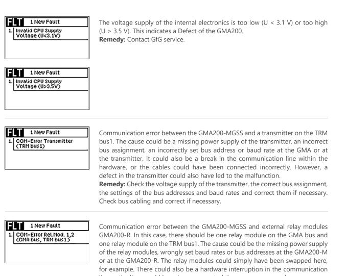
line or the lines could have been connected the wrong way round. **Remedy:** Check the power supply of the relay modules, correct device assignment, the setting of the bus addresses and baud rates and set them correctly if necessary. Check bus cabling and correct if necessary.
