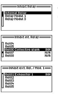
One or more relays can be inhibited for maintenance purposes (INH = Inhibit).
