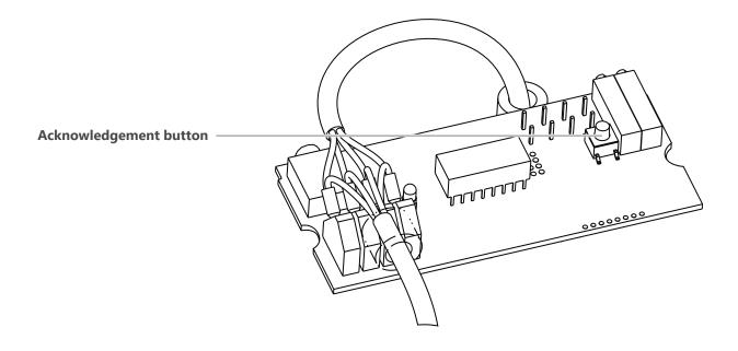
To do so, remove the cover and the housing lid and briefly press the acknowledgement button on the circuit board.
