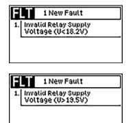
If the GMA is **only supplied by the PC via the USB cable** for configuration, the message "Inadmissible relay supply voltage (U < 18.2 V)" is always displayed together with the message "Inadmissible GMA supply voltage (U < 20 V)". This is normal.
