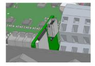
The GMA200-MGSS has a USB port and a slot for a microSD card on the motherboard. These are located to the left of the relay terminal block.
