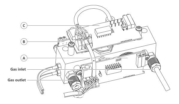
The GMA200-MGSS has an internal sensor block. This sensor block is configured at the factory according to the specifications at the time of ordering and is delivered fully assembled.
