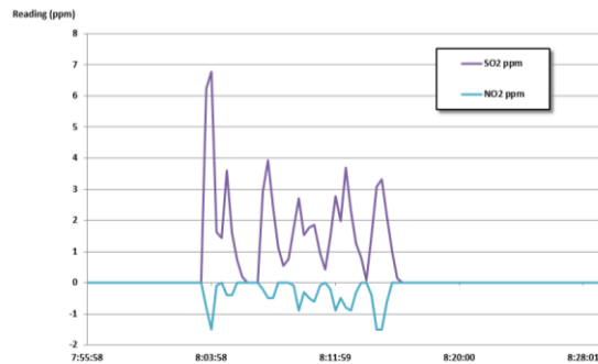
G460 instrument #3, readings from coal seam vent, SO 2 and NO 2
