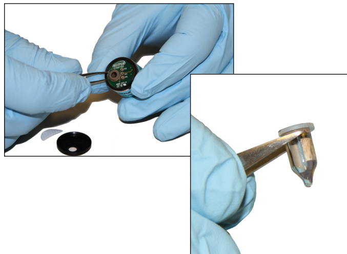
Figure 8: PID components showing detector body and lamp.
