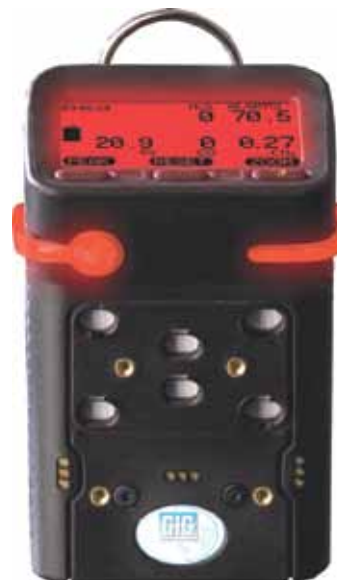
Portable multi-sensor landfill gas monitors can be equipped with standard pellistor LEL, NDIR combustible gas, NDIR CO 2 , PID and a wide range of other sensors for the direct measurement of toxic gases
