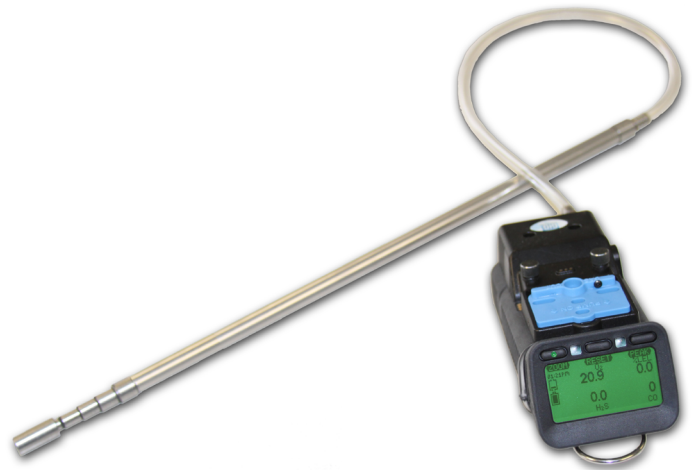
Figure 18: Sampling inerted vessels often requires very long sample lines. Use of an attachable motorized sampling pump allows the G460 from GfG Instrumentation pictured above to be located up to 300 feet away from the point where the sample is obtained.
