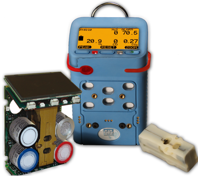
Figure 6: Instrument with NDIR sensor. Since the amount of IR light absorbed is proportional to the amount of target gas present, the longer the optical path-length through the IR sensor, the better the resolution.
