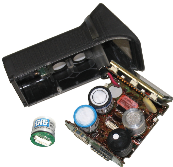
Figure 2: Multi-sensor instruments are able to use a wide range of sensors and detection technologies including \text{O}_2 , standard pellistor LEL, NDIR combustible gas and \text{CO}_2 , PID and over 20 different substance-specific electrochemical sensors for toxic gas measurement.
