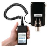
sensors are therefore installed near the simplify servicing, these ceiling. To transmitters can be equipped with a permanently installed cable meaning that the RC2 remote control can be connected for maintenance work and settings can be made from ground level. The display of the RC2 remote control shows the same information as would be shown by the EC28 versions with a display. This makes inspection, maintenance and calibration much easier.
